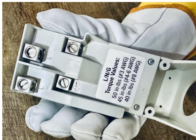
Figure 37 – Connection Module Terminals.
