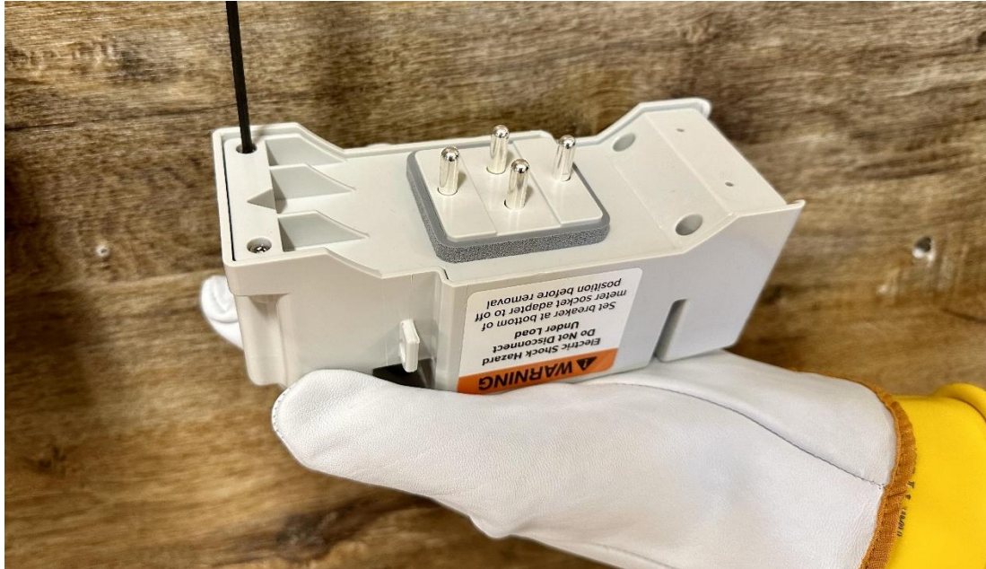
Figure 33 – Torque the Connection Module Screws.
