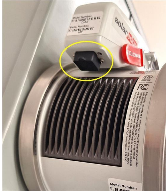
Figure 33. Ethernet RJ-45 Port. Remove Dust Cap for Cable Connection.
