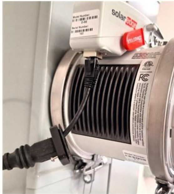
Figure 34. Mate the Ethernet Cable to the Communications Module RJ-45 Port.
