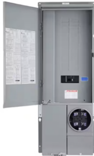
Figure 13. Top Door Combination Meter Socket / Load Centers. Once the Connection Module is installed on top of the MSA Base, IF it inhibits access to the service disconnect / breaker enclosure, this meter socket is NOT suitable for an MSA installation.
