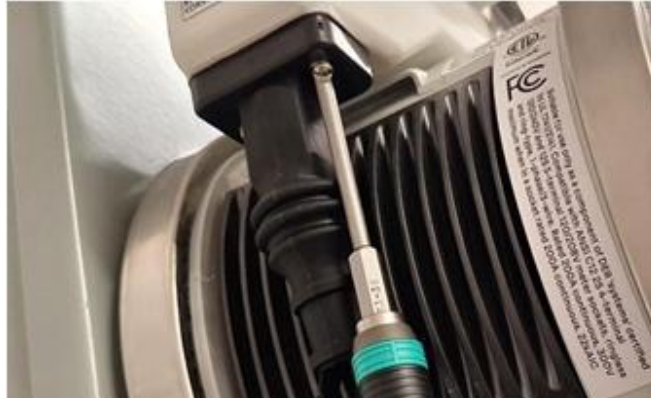
Figure 35. Torque Boot Assembly Screws to 2 in. lbs.
