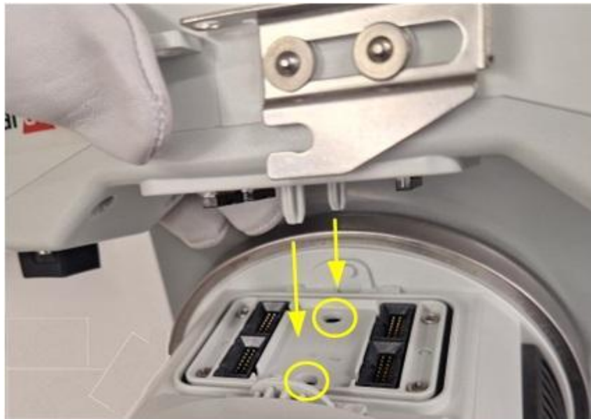
Figure 25. Insert the Connection Module.
