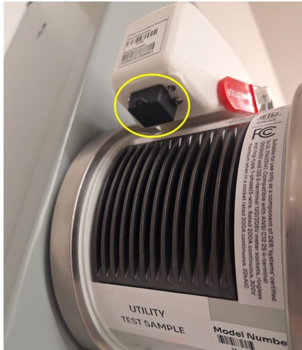
Figure 30 – Ethernet RJ-45 Port Capped Off.
