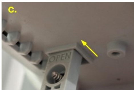
Figure 53 – Manual MID Override Switch Closure Procedure.
