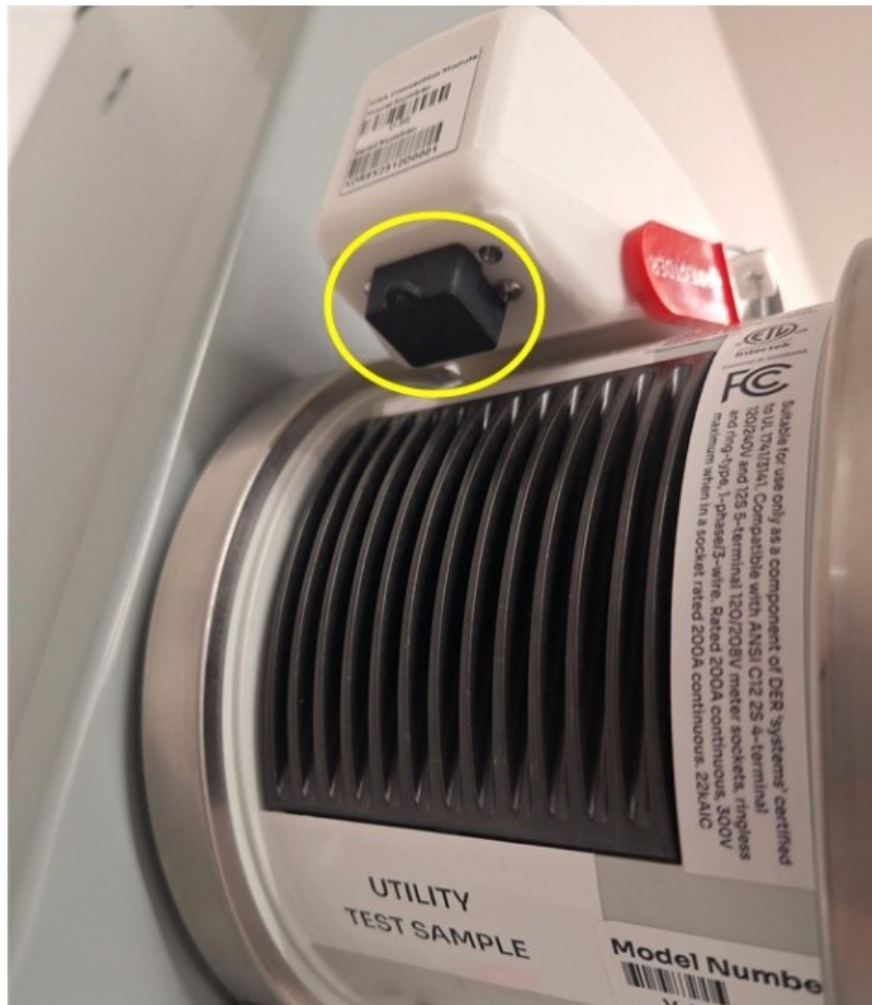
Figure 43 – Ethernet RJ-45 Port Capped Off.
