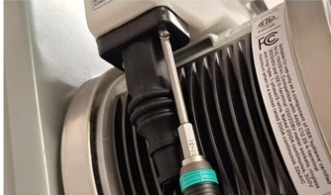
Figure 45 – Torque Boot Assembly Screws to 2 in. lbs.
