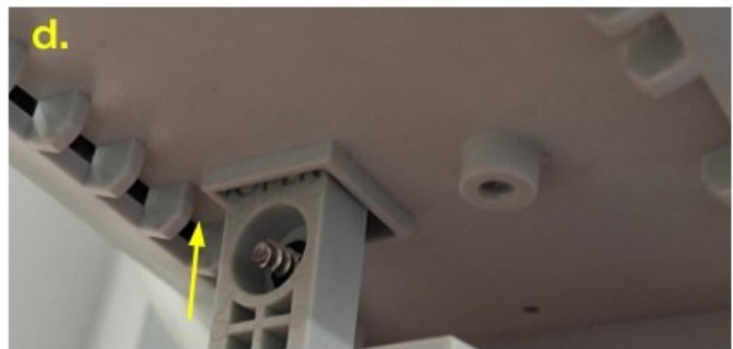
Figure 53 – Manual MID Override Switch Closure Procedure.
