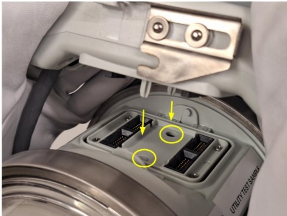
Figure 26 – Insert the Connection Module.
