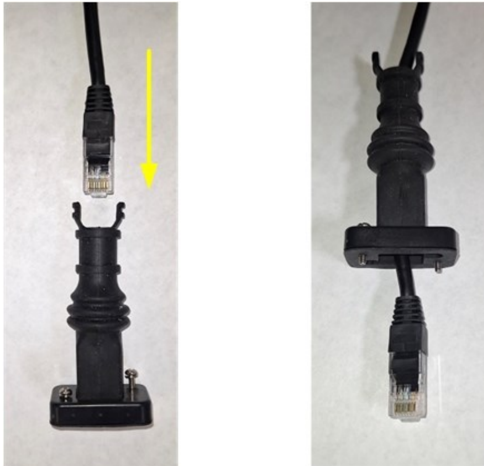
Figure 42 – Ethernet Cable Through Boot and Cover Plate.
