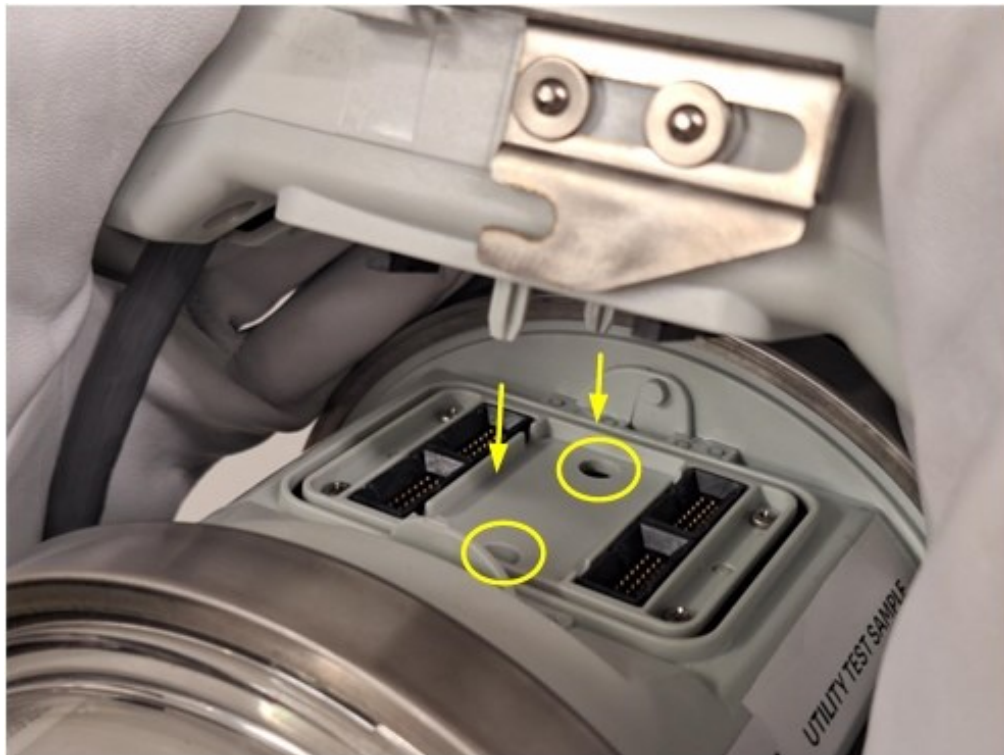
Figure 35 – Insert the Analog Connection Module.
