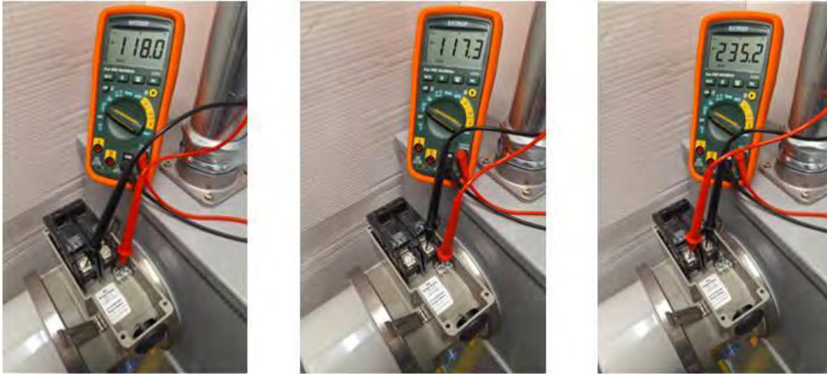
Figure 25 – Verify Voltage at Junction Box
