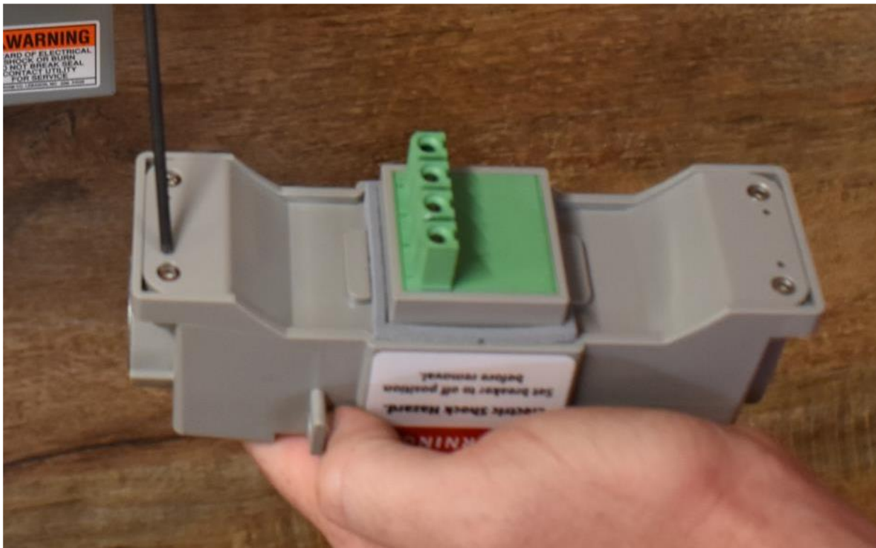
Figure 28 – Torque the Junction Box Screws
