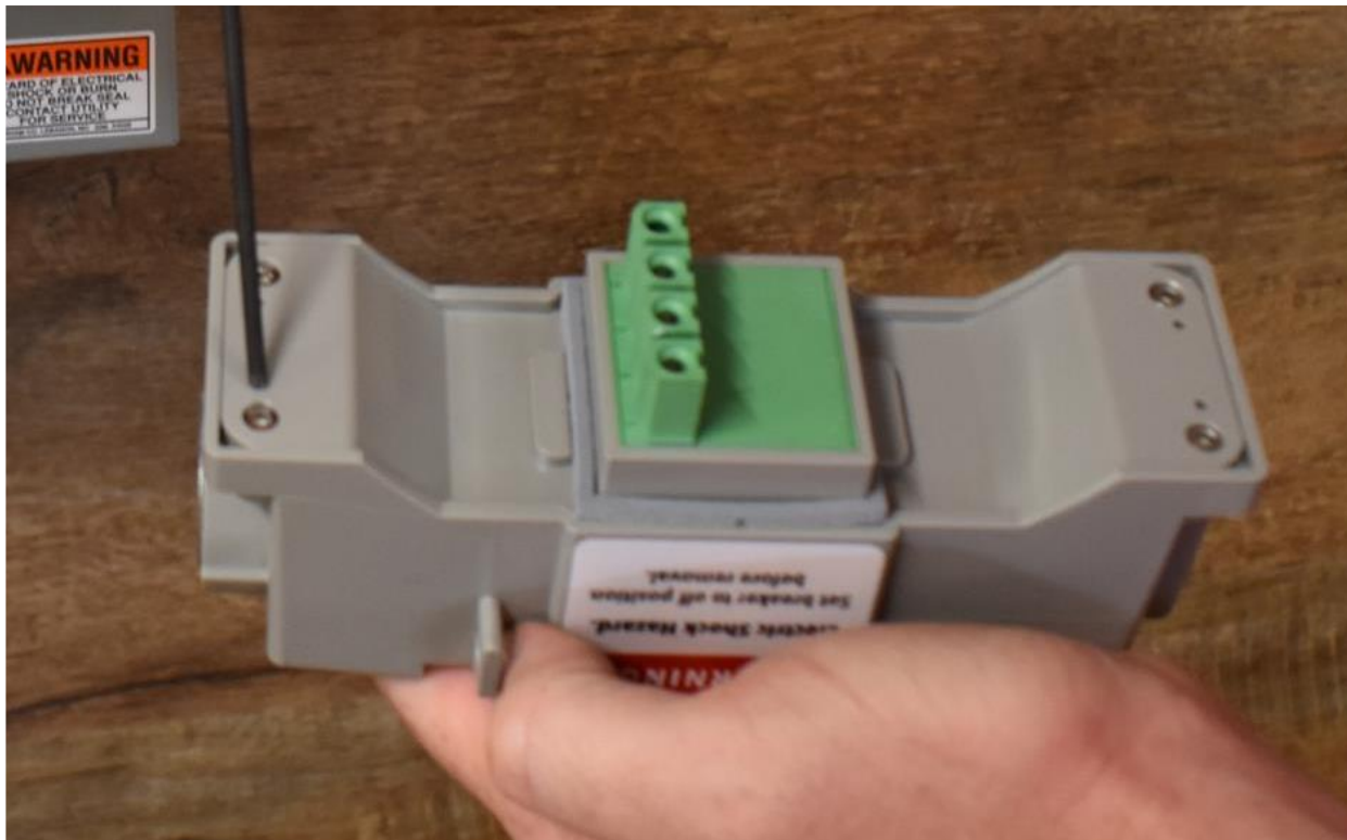
Figure 21 – Torque the Junction Box Screws
