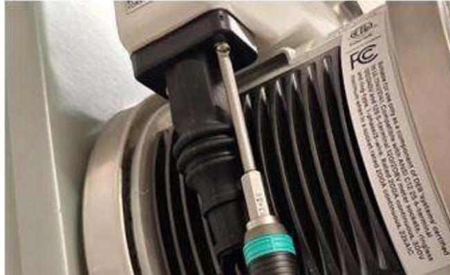
Figure 35. Torque Boot Assembly Screws to 2 in. lbs.
