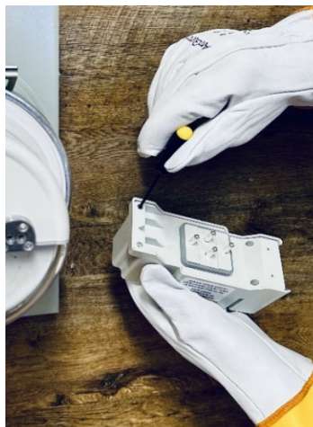
Figure 37. Connection Module Removed from the MSA Base.
