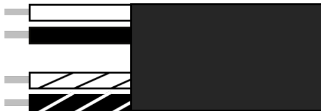
Figure 44. The non-terminated end of the CT Output Cable. The jacket has been stripped to expose the four conductors.
