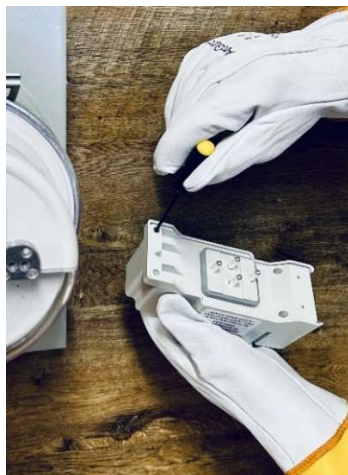
Figure 37. Connection Module Removed from the MSA Base.
