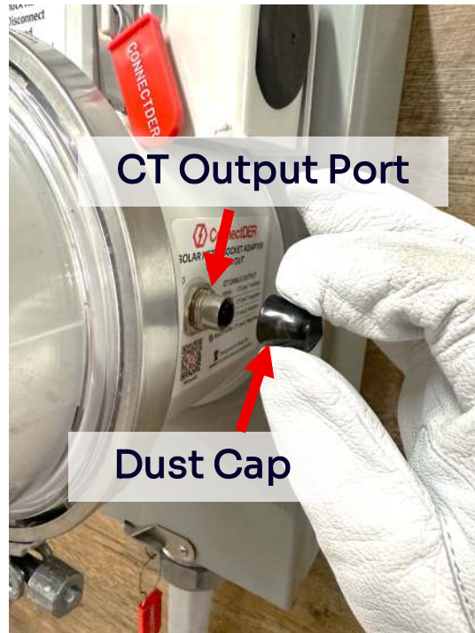
Figure 46. The CT Output Port can be found on the right side of the MSA Base.
