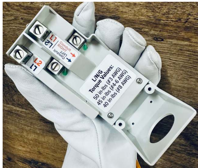
Figure 38. Connection Module Terminals. The colored L1/L2 labels provide additional guidance for landing the lines depending on if the conduit entry will be on the right or left.
