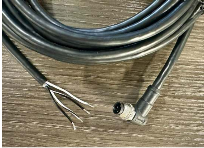
Figure 43. The CT Output Cable provided with Solar MSA V5.2 Data Out. Left: Non-terminated end (lands in the inverter). Right: Terminated end (plugs into MSA).
