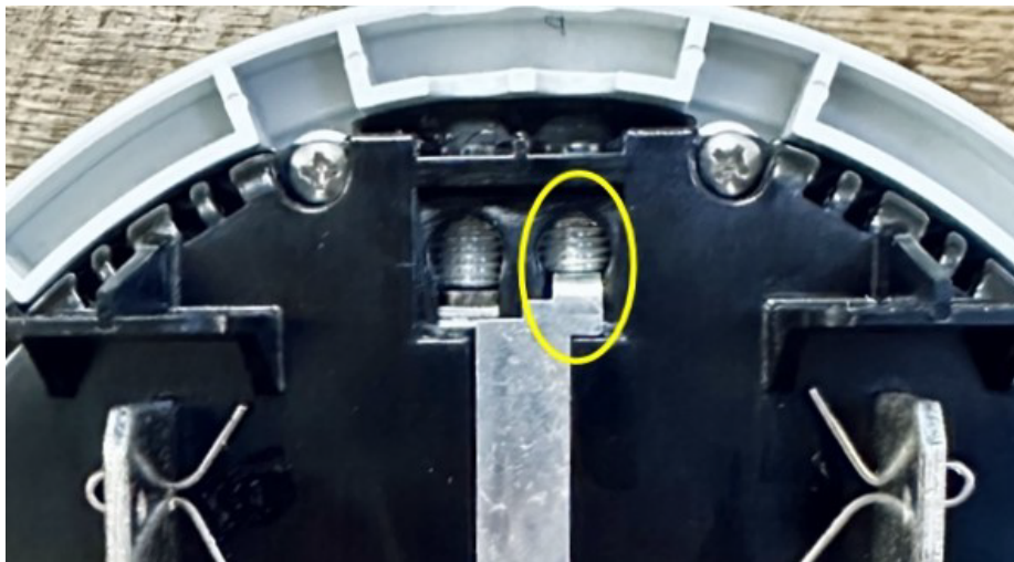
Figure 18. 5 th Stab Inserted to the back of the Solar MSA Base.
