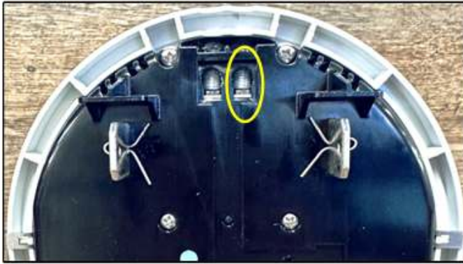
Figure 17. Loosen the Right-Side N/G Screw.
