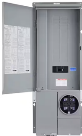
Figure 13. Top Door Combination Meter Socket / Load Centers. Once the Connection Module is installed on top of the MSA Base, IF it inhibits access to the service disconnect / breaker enclosure, this meter socket is NOT suitable for an IslandDER MSA installation.
