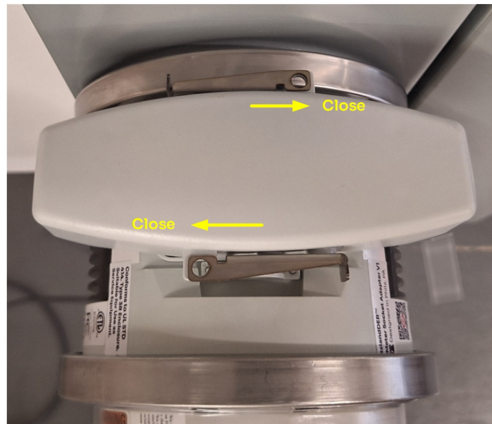
Figure 26. Slide the latches closed.
