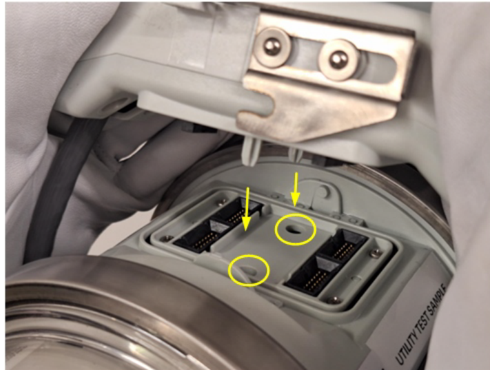
Figure 33. Insert the Connection Module.
